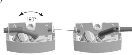
Optional: Install the pressure outlet on the right-hand side
