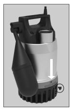
The pump housing is automatically vented. If this is not desired, the ventilation opening can be closed, e.g. for mobile operation.
