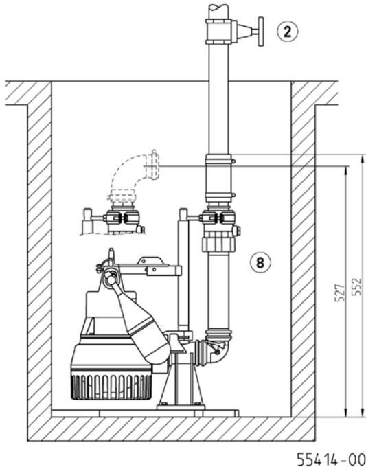
Example of installation and dimensions Easyfix 32 Duo (mm)
