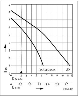
Specifications can be changed without notice. Performance subject to ISO 9906 tolerances. The minimum flow velocity in the pressure piping must be 0.7 m/s according to EN 12056. This data is represented in the performance curve as a limit of application.
